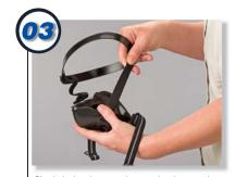
Check the headstraps to be sure they have not lost their elasticity. Make sure the straps are not
