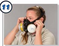
lighten the upper head straps in small, equa increments to ensure the top half of the respirator is tightened evenly and centered on your face.
