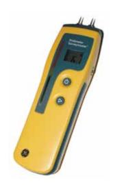
The Surveymaster is used for moisture measurement in buildings. Excessive moisture in buildings will lead to decay and deterioration of components and decorative finishes. Professionals involved with the identification, management and remedy of dampness need tools that help them to:
