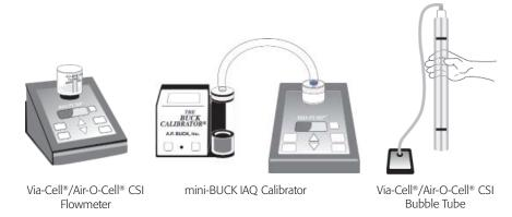
The Via-Cell flowmeter used with the Zefon Bio-Pump® has the in-line resistance of a sampler built into the calibration scale. When using the mini-BUCK or Via-Cell/Air-O-Cell CSI bubble tube, actual samplers are used in-line during calibration. For complete calibration instructions, please refer to the instructions included with your pump or calibration device.
