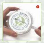
Remove the red plug and attach the sampling pump
