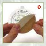
Peel the backing off of the label and stick it back onto the **BioCassette**, disconnect the pump, and reattach the red plug.
