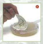
Peel off the **BioCassette** label and turn the sampling pump on for the desired sampling time.
